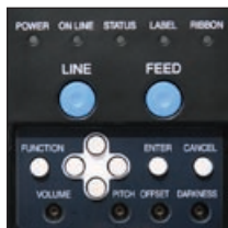
Multifunction buttons providing easy-to-navigate menu options
