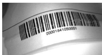
Figure 23 - Barcode Printed on Curved Surface Readable by Matrix 210N in spite of Image Optical Distortion
