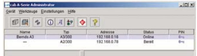
The cab network administration enables the administrator to manage all printers connected to one network at the same time. With a single mouse click different printers can be monitored, configured or updated with firmware; furthermore PIN codes of the printers are changed and data on the memory card can be managed.
