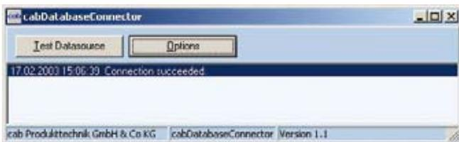
The cab database connector allows to link up stand-alone printers via TCP/IP interface to central SQL databases in the network. Data can be requested, printed and written back during the printing-process.
