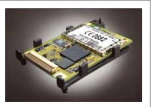
In control mode, the GSM module acts as a modem, allowing the UPS to be called from a distance and then executing information polling in order to verify its operating status at regular intervals and to carry out programming via SMS or data connection.
