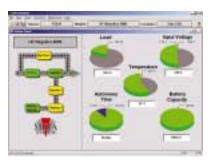
Our optional UPS SuperviSor shutdown software is available on CD-Rom and is able to manage the controlled shutdown of any operating system in heterogeneous network environments (Windows, Novell, Linux, most Unix).
