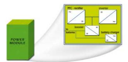
Each MegaLine power module is a true, on line dual conversion, with PFC rectifier - inverter - booster and battery charger. All the blocks of all the modules are in parallel, as are the batteries.
