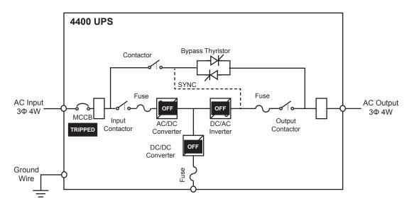
FIGURE 12-2 - EFFECT OF EPO ACTIVATION
