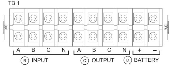
FIGURE 9.6 - 50KVA POWER CABLING LUGS
