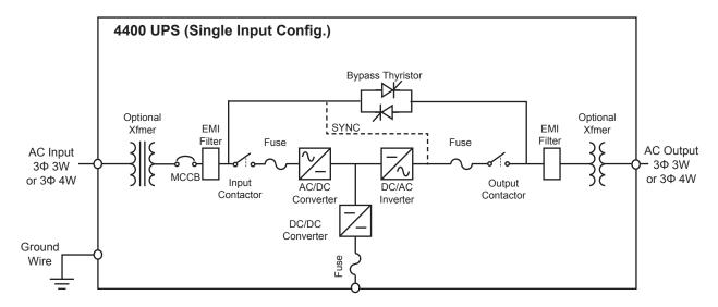
FIGURE 9.1 - 4400 SINGLE INPUT ONE-LINE DIAGRAM
