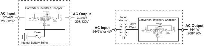
3. 4000 - WITH INTERNAL BATTERIES (15-50KVA)
