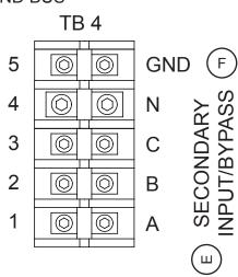
FIGURE 9.5 - 15-30KVA POWER CABLING LUGS
