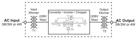
5. 4400 WITH INPUT AND OUTPUT TRANSFORMERS (15-50KVA)
