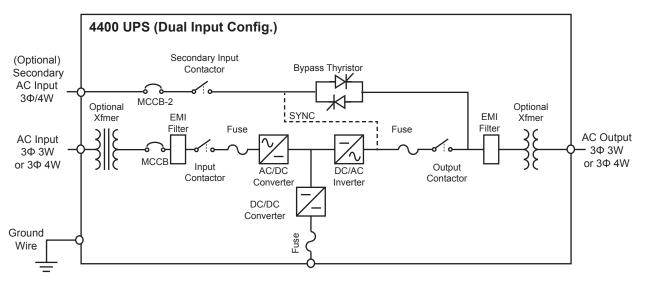
FIGURE 9.2 - 4400 DUAL INPUT ONE-LINE DIAGRAM
