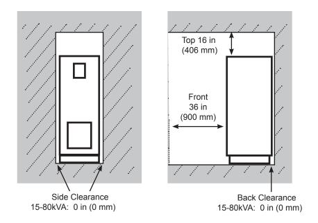
FIGURE 8.2 CLEARANCE FOR SEISMIC INSTALLATIONS
