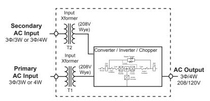
6. 4400 WITH DUAL INPUT TRANSFORMERS (15-50KVA)
