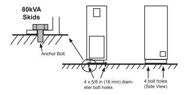
FIGURE 8.3 ANCHOR BOLT INSTALLATION DETAIL
