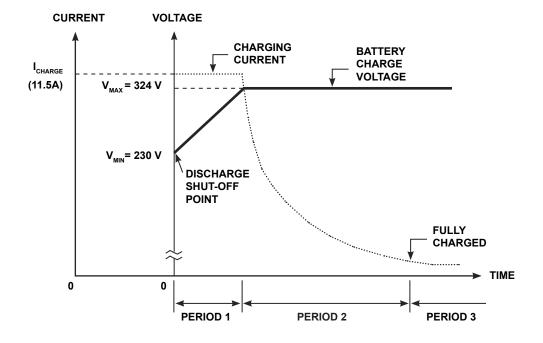
FIGURE 13.2 - TYPICAL BATTERY CHARGING CURVE
