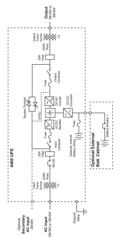
FIGURE 9.3 - ONE LINE DIAGRAM OF 4400 UPS WITH OPTIONAL MATCHING 4400 BATTERY CABINET
