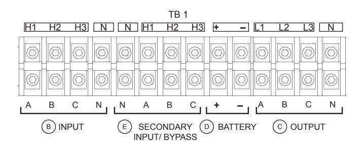
FIGURE 9.7 - 80-100KVA POWER CABLING LUGS
