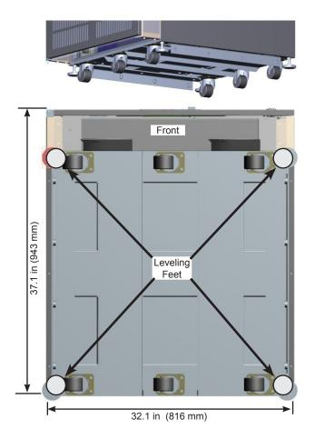
FIGURE 8.5 FOOTPRINT FOR 50 KVA USING LOAD LEVELING FEET
