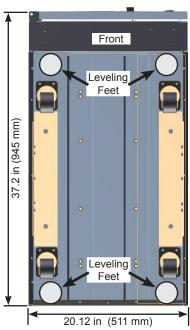
FIGURE 8.4 – FOOTPRINT FOR 15-30 KVA USING LOAD LEVELING FEET
