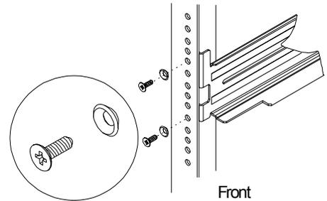
Align the bottom on the mounting rail with the bottom hole in the U-space (marked in step 3 above). Use the flat, Phillips head screws (10-32) and conical washers to attach the front rail to the rack. Position the rails so that the lip of the rail is on the bottom.
