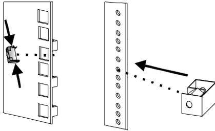
If your rack has round holes, insert clip nuts
