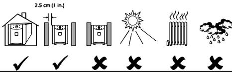
Install the UPS in a protected area that is free of excessive dust and has adequate air flow. Do not operate the UPS where the temperature and humidity are outside the specified limits.
