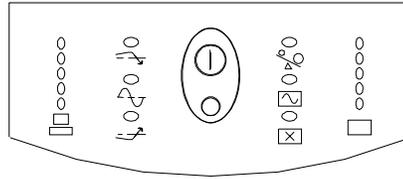
① With the UPS plugged in, press and release the large upper on/test button to supply power to the loads. The loads are immediately powered while the UPS beeps and performs a self-test.
